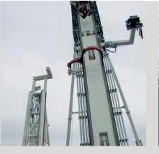
The central element of the camera system is the VISULEX Ex camera; this can either be mounted on a sight glass fitted to the reactor or set up outdoors (at a gate, tank depot, etc.) for monitoring property and plant.
