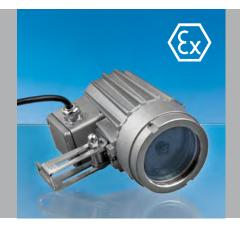
VISULEX Ex-Camera K06-Ex aluminium, with fixed lens II 2G Ex de IIC T6 Gb II 2G Ex the IIIC T80°C Db The lens of this camera is set during installation to focus on the property or object to be monitored. This can be an outdoor area, outdoor facility or part of a technical process. Maximum transmission
