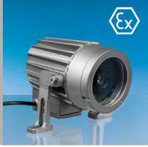
VISULEX Ex-Camera K07-Ex aluminium, with zoom lens II 2G Ex de IIC T6 Gb II 2G Ex tb IIIC T80°C Db The zoom lens of this camera is externally operated by remote control from the control room. The person monitoring can adjust any of the technical settings to meet his individual requirements.
