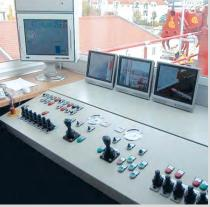
The captured images are transmitted to a screen in the control room by way of a cable which can be up to 500 m long.
